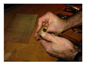
Start the shaping of the top piece by laying it against the end of the tube, then start bending the edges inwards.
