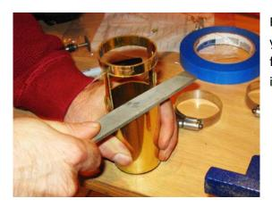
File and sand everything smooth. Brass is soft, so if you didn't cut things absolutely perfectly, a metal file and some elbow grease can fix a multitude of inaccuracies.
